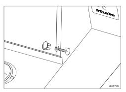
With grease filters removed, secure the range hood, or fit the side panels, using two screws per side.
